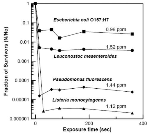
**Inactivation of food-transmitted microorganisms (vegetative cell in pure suspensions) by aqueous ozone**
